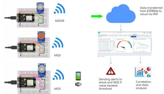
Fig. 5 Experimental Setup of the Air Quality real-time Monitoring device
